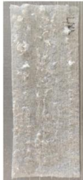
White ADL- Acquisition Distribution layer
